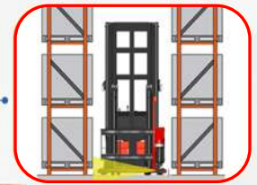
Fork camera & horizontal laser line to identify beam position
