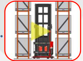
Judging left corner blind area and the space to the left and right of the pallet when picking up
