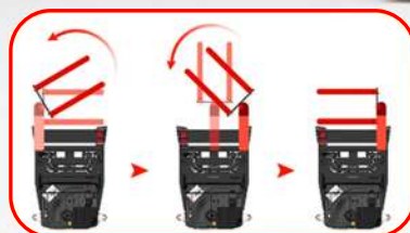
Fork rotation and side shift can be operated at the same time.
