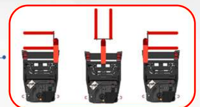
Active safety function: travel lock function
