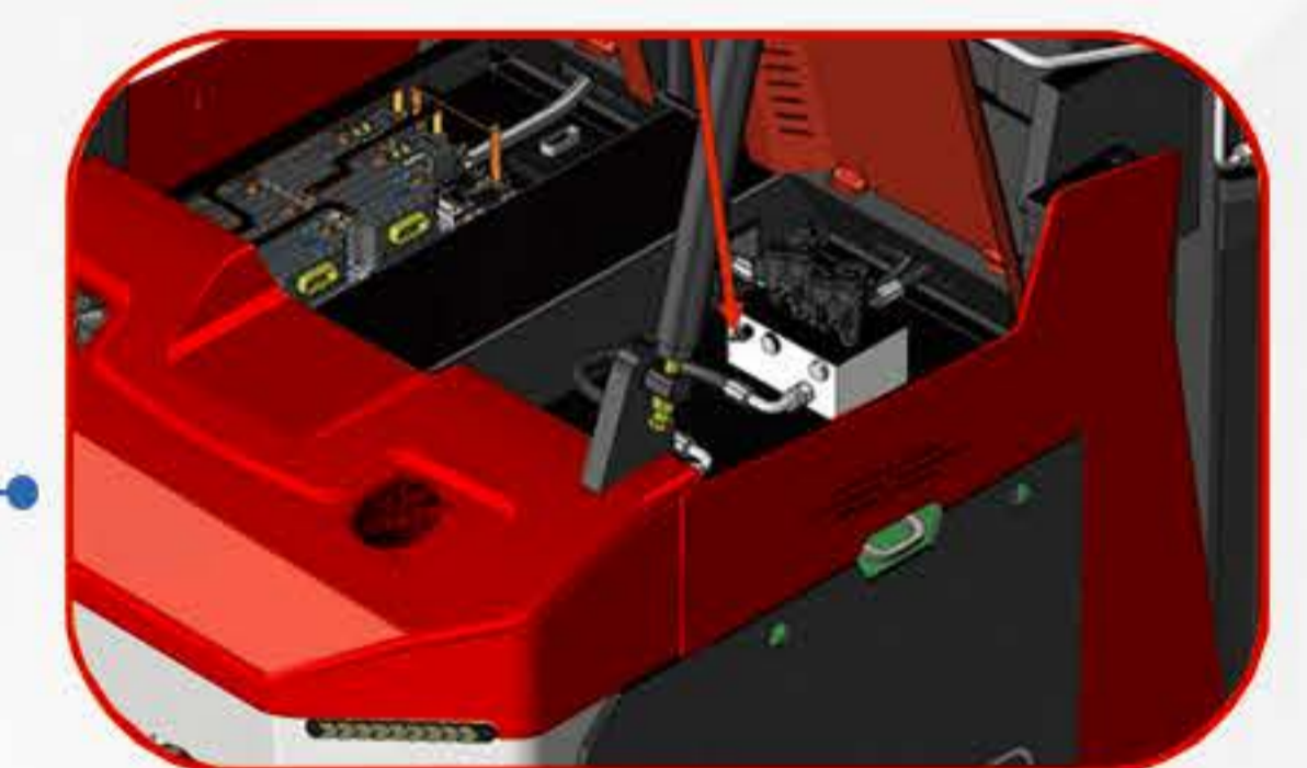
Emergency operation handle for quick lowering to the ground..
