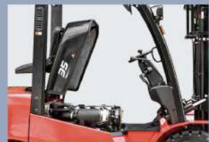
The wide-open hood, increasing maintenance space by 10%.
