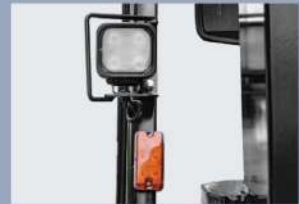
The LED lighting system is provided in the entire forklift, which can save energy and power and greatly improve the performance and service life of lights.
