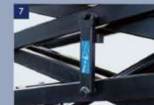
7 Supporting arms: To protect the operator when he is doing repair or maintenance job
