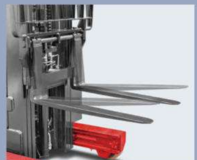
Forks can tilt forward/backward for easy loading
