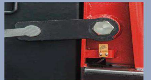
The locking device of the battery is provided with the safety protection function. Only if the locking device is rotated in place, the tractor can travel
