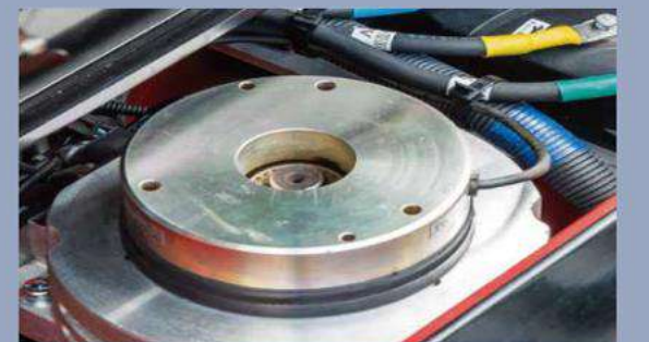
Electrical Park Brake (EPB) system
